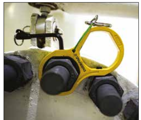
▼ Enerpac Back-Up Spanners to be used to stop the back nut from turning during make up or break out.
